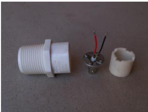
Fig. 12 - Masthead Base Subassembly
