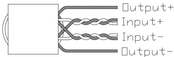
Fig. 6 - Construction Details for Transformer T2
