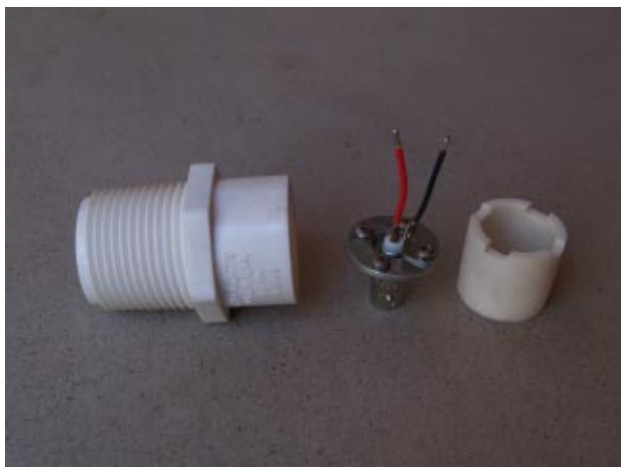
Fig. 12 - Masthead Base Subassembly
