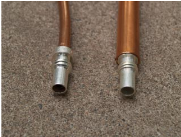
Fig. 14 - PL-259 Reducers Attached to 1/4" (left) and 1/2" (right) Copper Tubing
