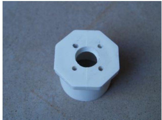
Fig. 9 - Machining Details for PVC End Plugs
