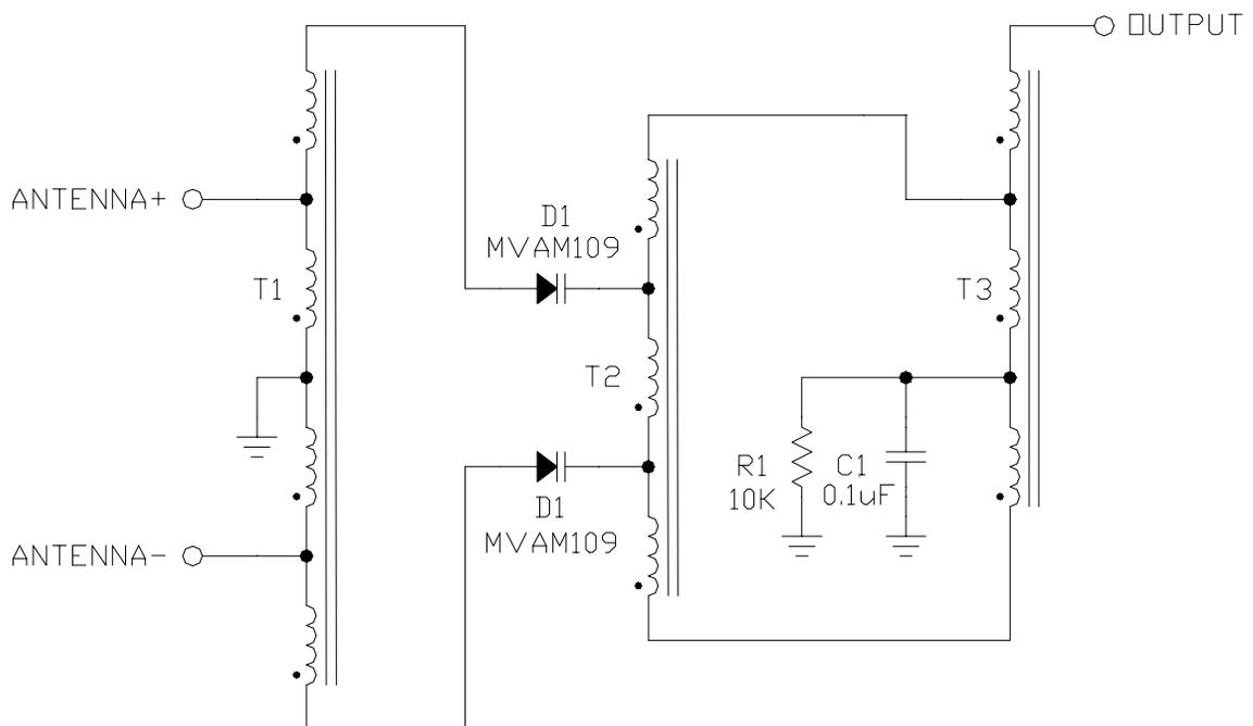
Fig. 4 - Varactor-Tuned Loop Antenna Matching Network Schematic
