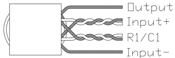
Fig. 7 - Construction Details for Transformer T3
